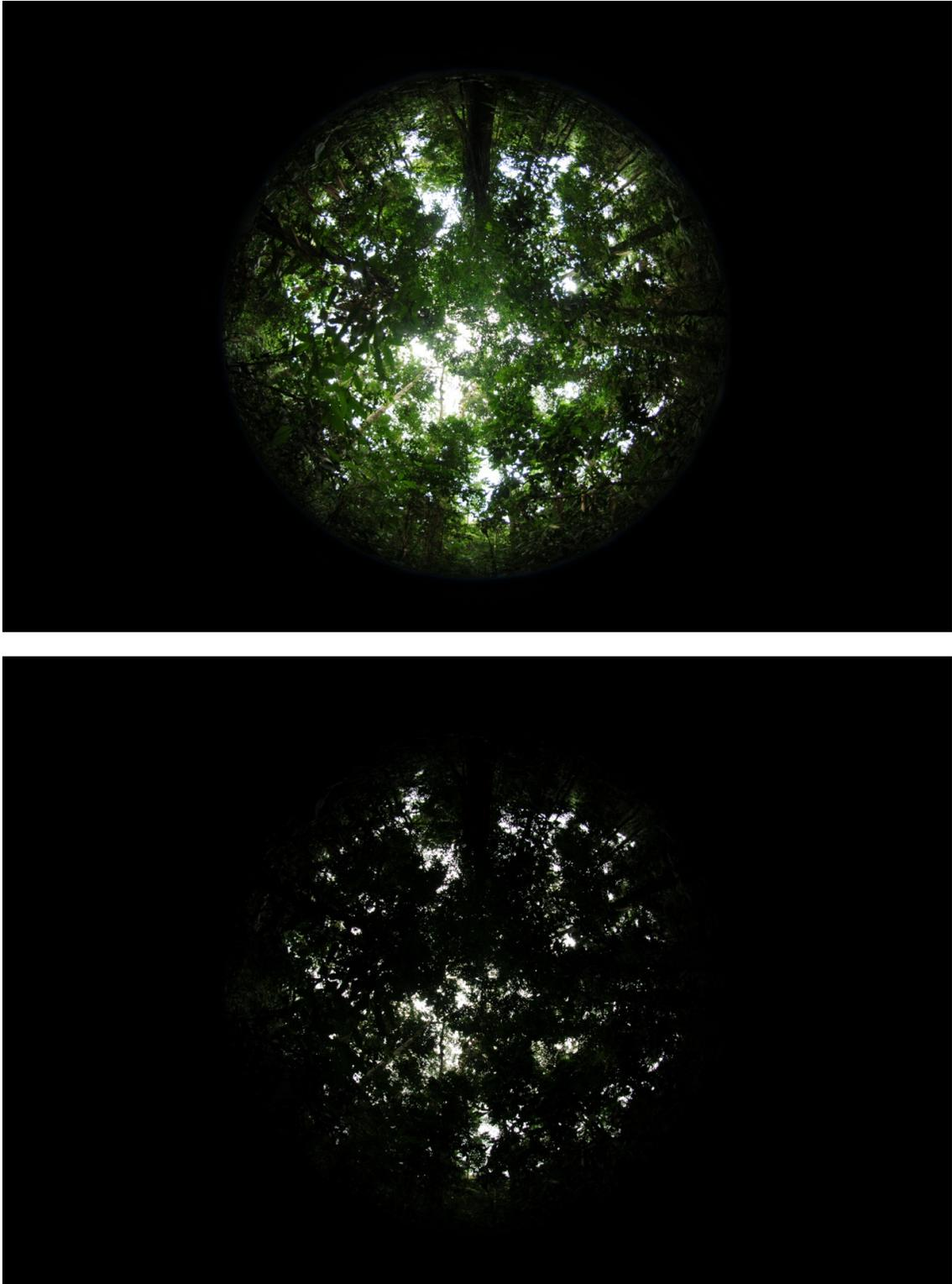
Figure 5: Example of hemispherical photograph (image from plot YAN/I, primary forest). Top: image acquired using standard exposure setting; Bottom: underexposed image.
